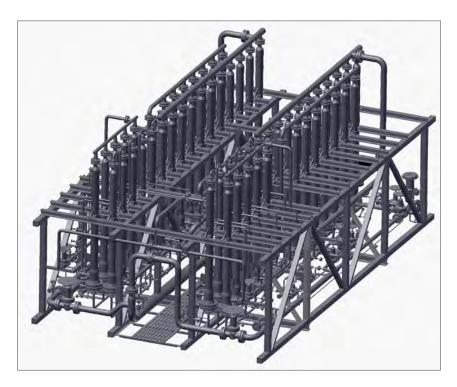
Typical oil refinery systems produce hydrogen with purities between 90 to 98 mol%. Product gas purity is dependent upon feed composition, available differential partial pressure and required hydrogen recovery level. The hydrocarbon-rich stream is returned at nearly the same pressure as the feed gas for use as fuel gas.
