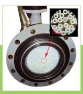
A PRISM Membrane separator contains thousands of fibers, which are bundled and encased at one end in epoxy resin. The bundle of fibers is inserted in a coded pressure vessel to provide correct flow distribution and pressure segregation.
