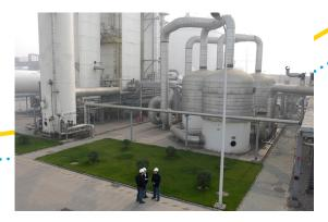
Remove H<sub>2</sub>O, CO<sub>2</sub>, N<sub>2</sub>O and hydrocarbons
