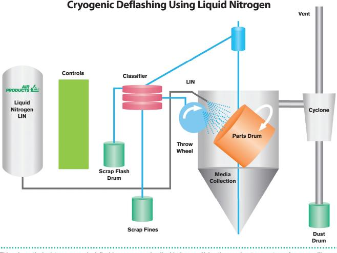
This schematic depicts a cryogenic deflashing process using liquid nitrogen. Using the very low temperature of cryogens like liquid nitrogen, cryogenic deflashing temporarily embrittles residual material for removal when subjected to stress applied though tumbling and media blasting.
